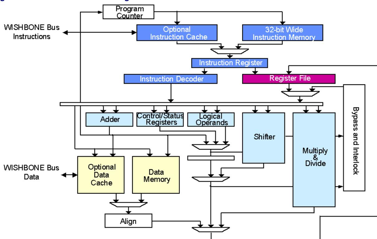
To accelerate the development of processor systems, several optional peripheral components are available with the LatticeMico32 processor. Specifically, these components are connected to the processor through a WISHBONE bus interface, a royalty-free, public-domain specification. By using this open source bus interface, you can incorporate your own
