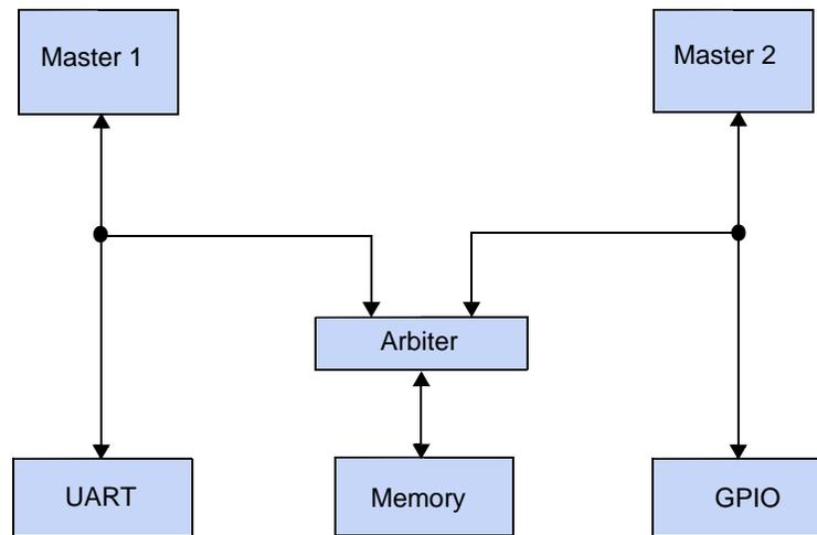
In slave-side arbitration, each multi-master slave has its own arbiter. A master port never waits to access a slave port, unless a different master port attempts to access the same slave port at the same time. As a result, multiple master ports active at the same time simultaneously transfer data with independent slave ports.
