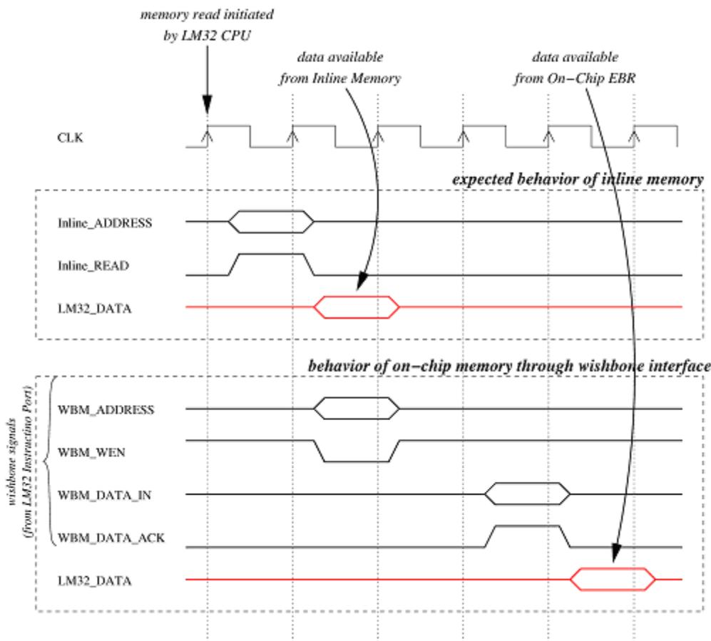
This diagram compares the number of cycles it takes to service read access from the LatticeMico32 CPU by the inline memory versus the Wishbone-based on-chip EBR. The read access initiated to inline memory will be completed in the next cycle, whereas a read access initiated to EBR will take four cycles. A similar behavior can be seen for writes initiated by the
