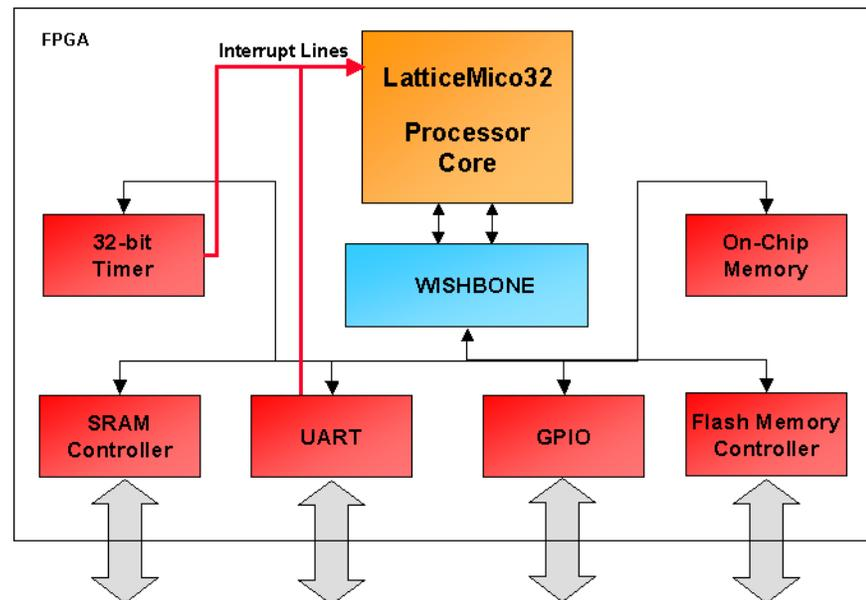
This manual describes the architecture of the LatticeMico32 processor. It includes information on configuration options, pipeline architecture, register architecture, memory architecture, debug architecture, and the instruction set. It is intended to be used as a reference when you design processors for use on supported Lattice Semiconductor field programmable gate arrays (FPGAs).
