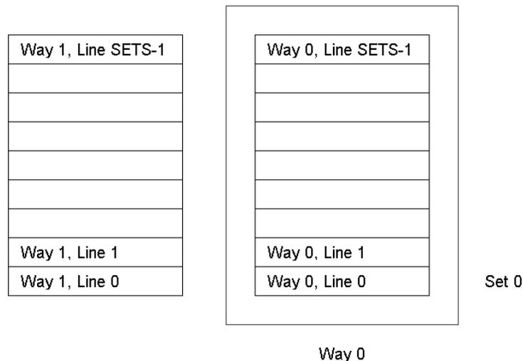
The LatticeMico32 caches are write-through, which means that whenever a store instruction writes to an address that is cached, the data is written to both the cache and main memory. A read-miss allocation policy means that a cache line is only fetched from memory for a load instruction. If a cache miss
